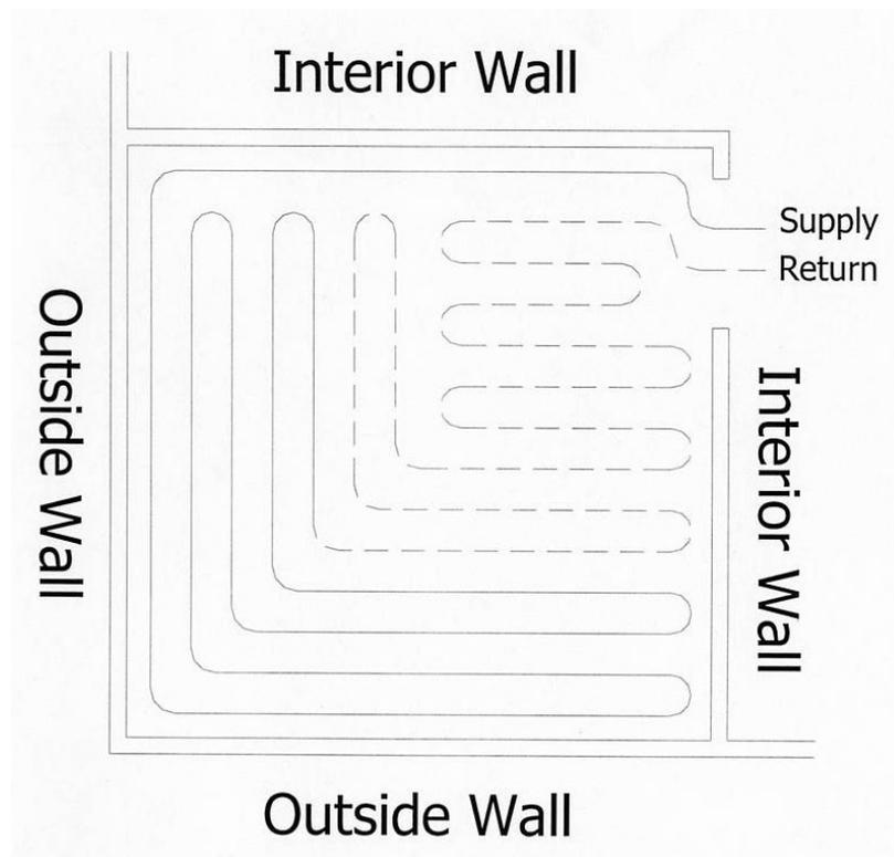
“There are a couple of ways for us to install the tubing. For new construction, we generally install the tubing over the sub-floor; we lay it out per the drawing, nail it down, and then cover it with either rigid foam insulation, called ThermalBoard, or a layer of lightweight concrete. This is the method you’ve seen used by the crew on “This Old House” when they install radiant heating.
